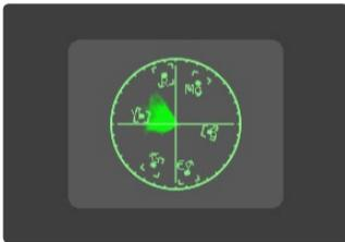
The Vectorscope duplicates the behavior of a specific type of video test equipment, displaying a circular graph that helps to visualize chrominance signals.
